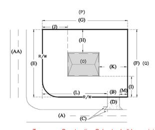
Temporary Construction Culverts shall be a minimum of 15" in diameter, unless otherwise specified by the Town Engineer. Failure to do so will result in a Red Tag fee that will be paid at the Lake Placid Government Center. If not addressed by the contractor/permittee within 15 days of the red tag notice, the Town of Lake Placid will remove the deficient temporary pipe and driveway.
